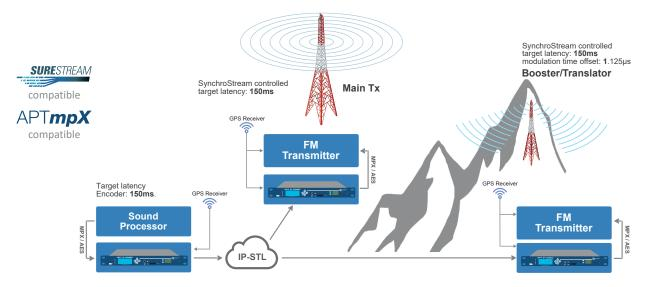
Transmission on a Single Frequency Network requires perfect compansation of IP-Link latencies and management of the modulation-timing
