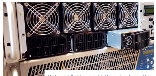
Redundant & Hot-swappable Power Supplies and Fans
