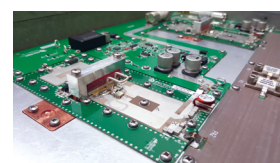
2 planar design RF pallets each of 1.25 kW
