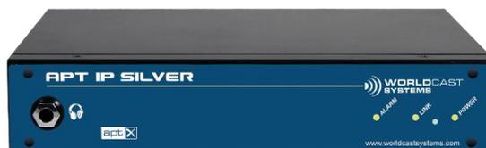
Add to this the variety of network functions: VLAN, IP aliasing, or the "Reply to Sender" NAT traversal mode - the APT IP Silver ensures it perfectly integrates into any network environment. In addition, it's optimized for use in mobile networks and offers serial AUX data transmission.
