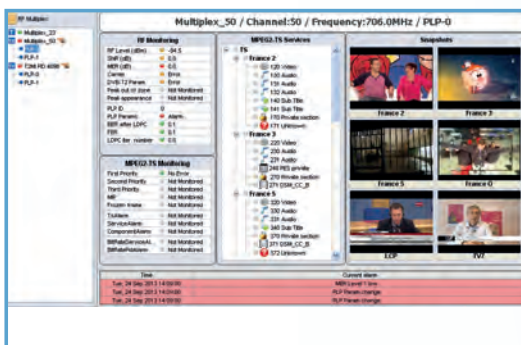
Status Page with Running Alarms
