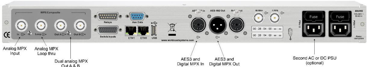
Figure 10: Shows all rear panel components of the MPX IP Codec
