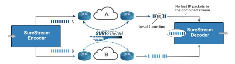
The figure shows the principle of SureStream. A network can be any data service, including wireless cellular networks.
