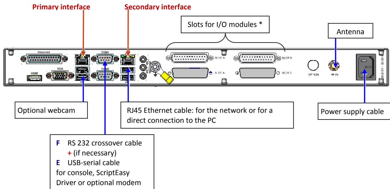
**i** With the current version only one serial port is enabled.
