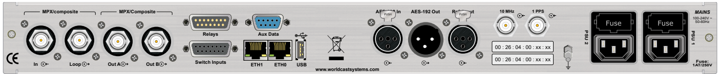
APT IP CODEC MPX rear panel. The illustration may deviate and show optional components.
